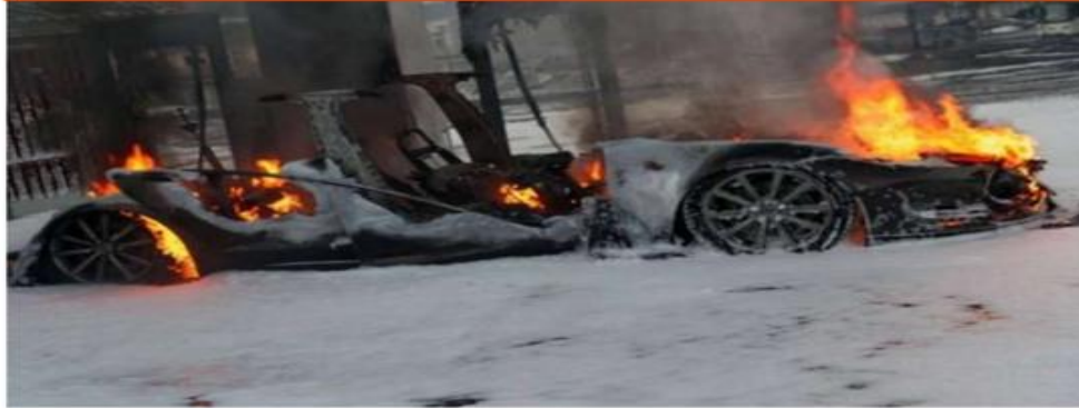
The fire on a Tesla Model S while being charged at the supercharging station in Norway on 1 January 2016, where the fire also spread to the passenger compartment
